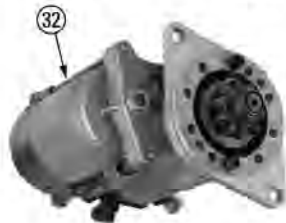
Gear Reduction "Super" Starter
