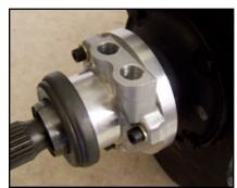
• If necessary use a small screwdriver to align the the slave cylinder holes with the holes in the bell-housing. Install the two fittings making sure that the shorter one is on the left and the longer one on the right and that they are tight.
