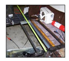
Mark the driver's floor board and cut out for clearance around the new pedal assembly. Reinstall the floor board.
